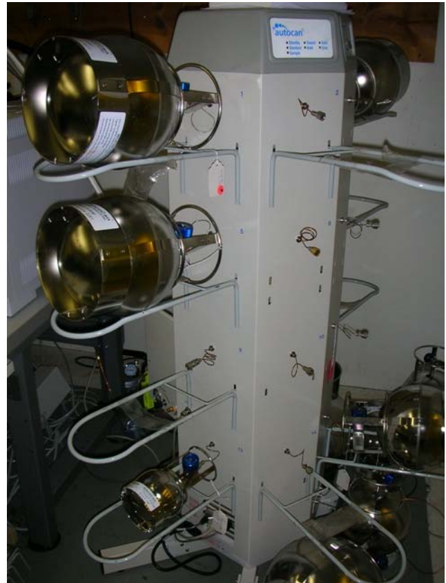
Figure 4: Autosampler for air sampling canisters. If threads on canisters are found to be cross-threaded or otherwise disturbed, the laboratory may not be able to secure a leak-proof seal between the canister and the autosampler connection point,
